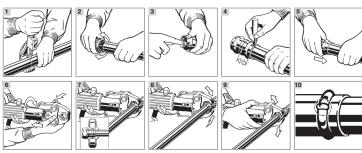
1 Cut stainless-steel tubing only with an approved stainless-steel tube cutting tool. Cut the tube square using a displacementtype cutter or fine-tooth saw.
