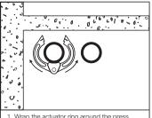
1. Wrap the actuator ring around the press fitting with the opening facing away from you.
