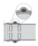
Fittings are radially pressed around the sealing element in a single step.
