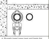
4. Properly insert press jaws and begin the press-fitting procedure.
