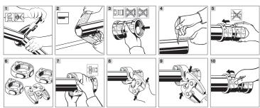
1 Cut stainless-steel tubing only with an approved stainless-steel tube cutting tool. Cut the tube square using a displacement-type cutter or fine-tooth saw.
