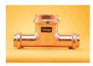
Viega ProPress may only be pressed onto copper tube in accordance with ASTM B88 or B75. When pressing onto B88 copper tube, types K, L, and M may be used. Tempers O60 and O50, known as "soft copper", are
