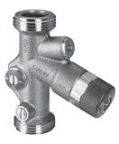
**Description** The ProPress automatic recirculation regulating valve provides automatic balancing of domestic hot water recirculation return lines. Balancing based on hot water return temperature allows the recirculation system to run more efficiently with smaller pipes and circulators.
