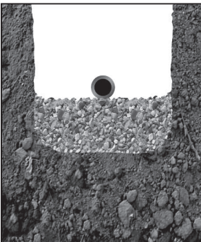
Trench in bad soil
