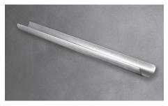
Viega PureFlow support trays are for use with clevis hangers and/or coated ring clamps to help reduce the number of support hangers required for hanging PureFlow tubing. These trays are available in 10 ft. lengths for ½" through 2" PureFlow tubing sizes.
