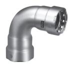
MegaPress 316 fittings are designed to be used with standard IPS ASTM A312 stainless steel pipe and are ideal for industrial applications. MegaPress 316 1/2" to 2" fittings can be used with Schedule 5 to Schedule 40 stainless steel pipe and 21/2" to 4" fittings can be used with Schedule 10 to Schedule
