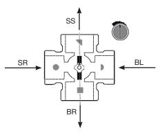
For precise temperature control it is imperative that the initial position of the valve used is half open. This can be accomplished by positioning the groove of the white plastic adapter between boiler supply and boiler return. The actuator itself can be mounted onto the valve in any position.
