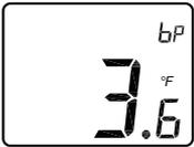
Sets the differential temperature of the proportional bandwidth with respect to how well insulated the house is. The better insulated the house, the smaller the bandwidth temperature required. This feature is only available if rEG regulation is selected in the J7 parameter. The default setting is 3.6°F. Other suggested settings:
