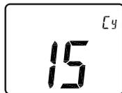
Proportional integral regulation time cycle value in minutes. This feature is only available if rEG regulation is selected in the J7 parameter. The default setting is 15 minutes and is recommended for radiant slab heating applications. Other possibilities are:
