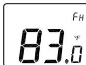
Adjust to set the floor temperature high limit. Adjustment range is 83°F to 99°F with 83°F being the default setting.
