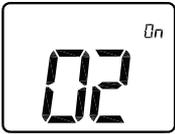
Minimal starting time in minutes. Adjustable from 0 to half of the cy parameter setting. Default is 02.
