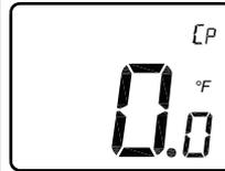
Adjust setting to match the current load of the device being controlled by the thermostat. If the current draw of the device being controlled by the thermostat is less than 2 amp. then adjust this value to match the value selected in bp parameter. If the amp. draw is greater than 2 amp. set this value to the actual amperage. This function is only available if rEG regulation is selected in the J7 parameter. The default setting is 0.0°F.
