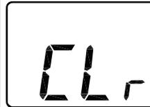
While in this parameter press and hold the OK button until the thermostat restarts to restore all factory defaults to thermostat.
