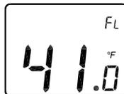
Adjust to set the floor temperature low limit. Adjustment range is 41°F to the FH setting. The default is 41°F.
