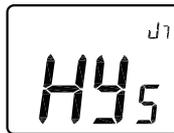
Select rEG for proportional band regulation of thermostat or HYs for the thermostat to operate on a static differential of 0.3°K. If HYs is selected Cy, bp, and Cp parameters become non-functional and require no settings. rEG is the factory default setting.
