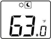
Places thermostat in reduced temperature operation indefinitely. Returning to Comfort Operating Mode takes thermostat out of Reduced Mode.
