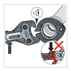
NOTE! Before initiating a press make sure the ball heads sit correctly in the contact points of the press ring.
