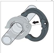
Open the press ring and place it around the pressing point on the press fitting.
