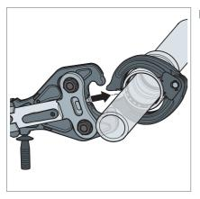
Place the open Viega Z3 actuator onto the press ring by inserting the ball heads of the actuator into the contact points of the press ring.
