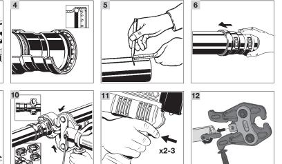
Mark proper insertion depth. Improper insertion depth may result in an improper seal. It is recommended that the depth marking be visible on the completed assembly.
