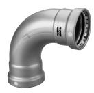
MegaPress 316 FKM fittings are designed to be used with standard IPS ASTM A312 stainless steel pipe to form a complete press system that is ideal for industrial applications. MegaPress 316 FKM ½" to 2" fittings can be used with Schedule 5 to Schedule 40 stainless steel pipe and
